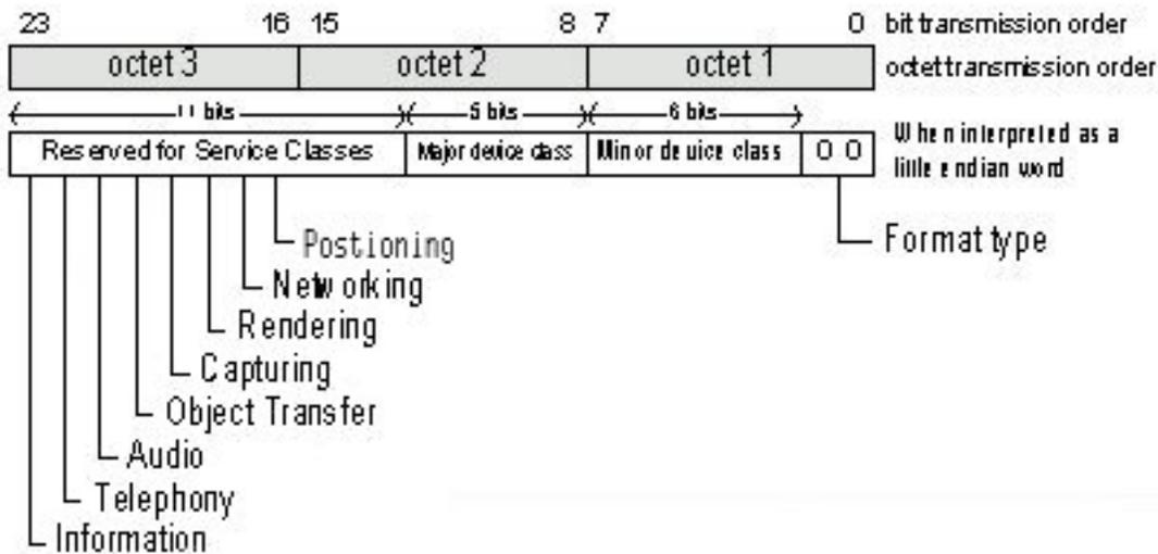
**Figure 1:** The Class of Device/Service field (first format type). Please note the order in which the octets are sent on the air and stored in memory. Bit number 0 is sent first on the air.
